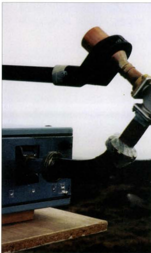
Fig. 6: A close-up shot of the waterpipe feed horn on the offset arm.
