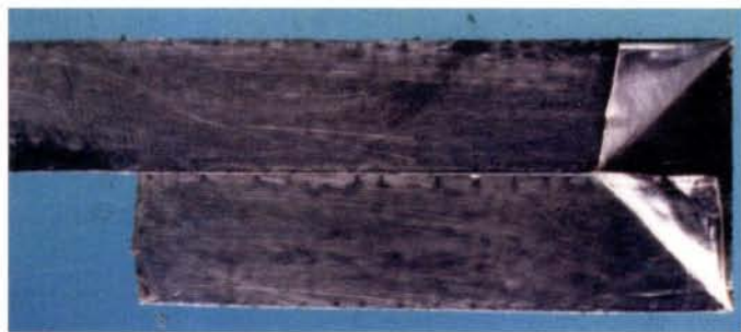
Fig. 5: Making a 'double' corner allows the tape width to be effectively increased.
