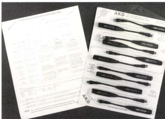
Fig. 1: Stevenage-based AKD have many years of experience in producing in-line filters suitable for helping to eliminate TVI. Allan Wightman used one to tackle problems experienced by G3XFD.
